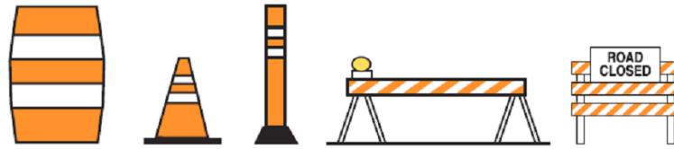
Barrel Cone Tube Barrier Road Closed
