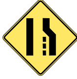
Lane Ends Merge Left
